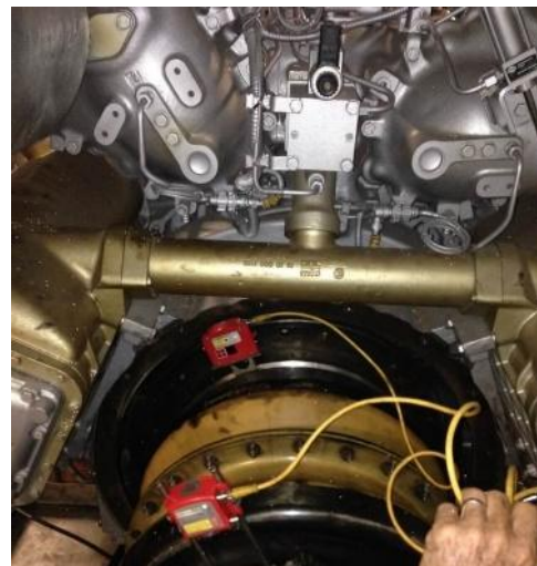
Figure 4 – Shaft alignment on Vessel x
