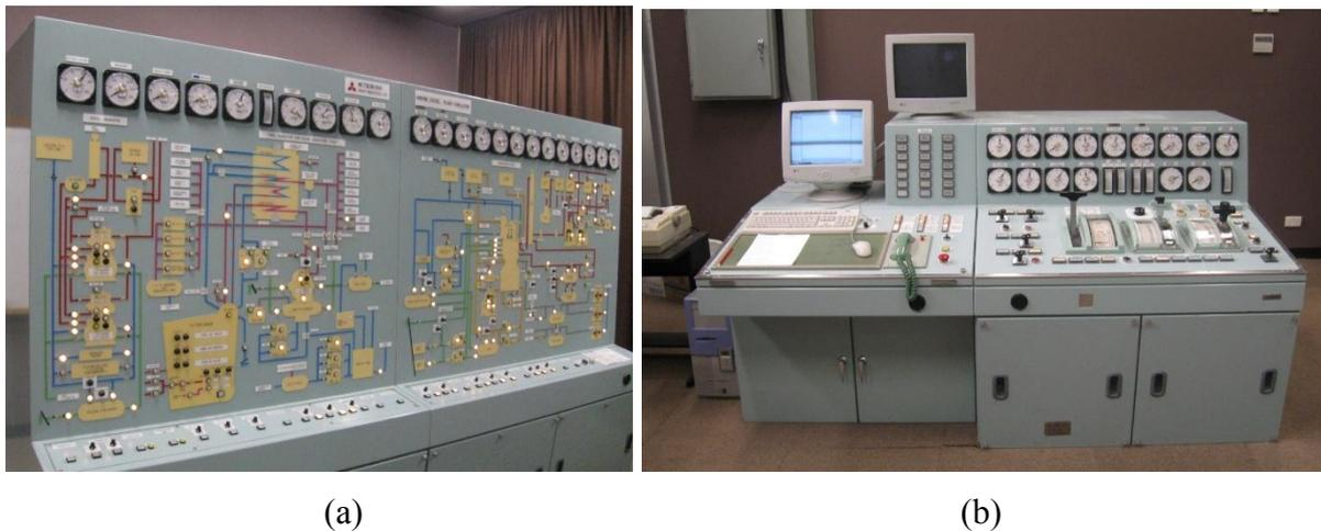
Figure 1. (a) Hardware based Engine Simulator installed at AMC in 1985, showing the entire engine room and the machinery space analogue mimic panel, (b) Engine Control Room console.
