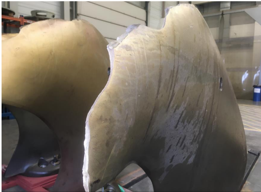
Image 4.1 Mechanical damage of the blade. Author's photograph.
