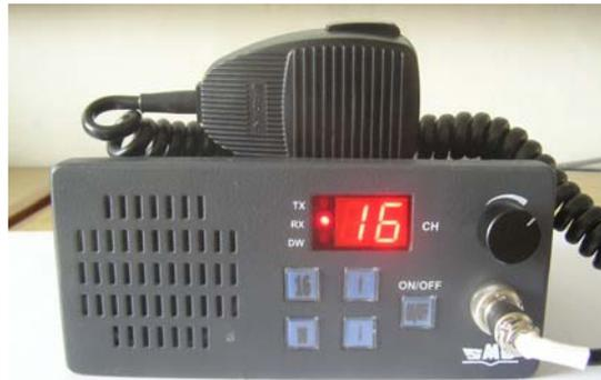
Fig. 3 Simulated VHF terminal
