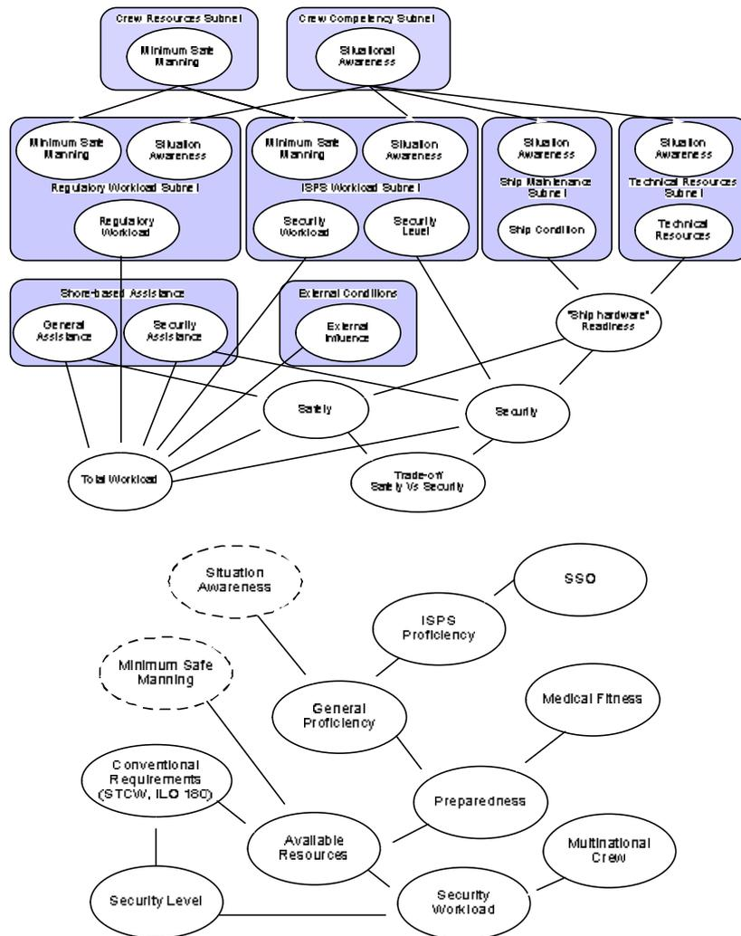
that enable an understanding of the failure mechanisms. It thus gives a quantified result whenever one of the input parameters is altered. In other words, each node could be identified as a Risk Control Measure (RCM), and their influence on safety and security could be monitored.
