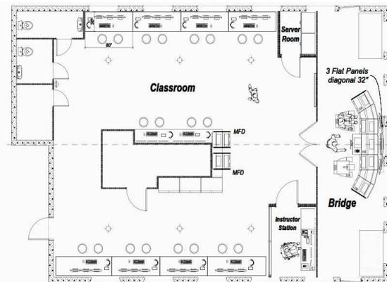
Figure 2 NavLab Layout
