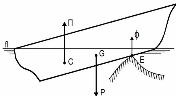
Figure 1 A ship grounded in point E
