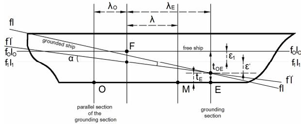
Figure 2 Forces acting on a grounded ship
