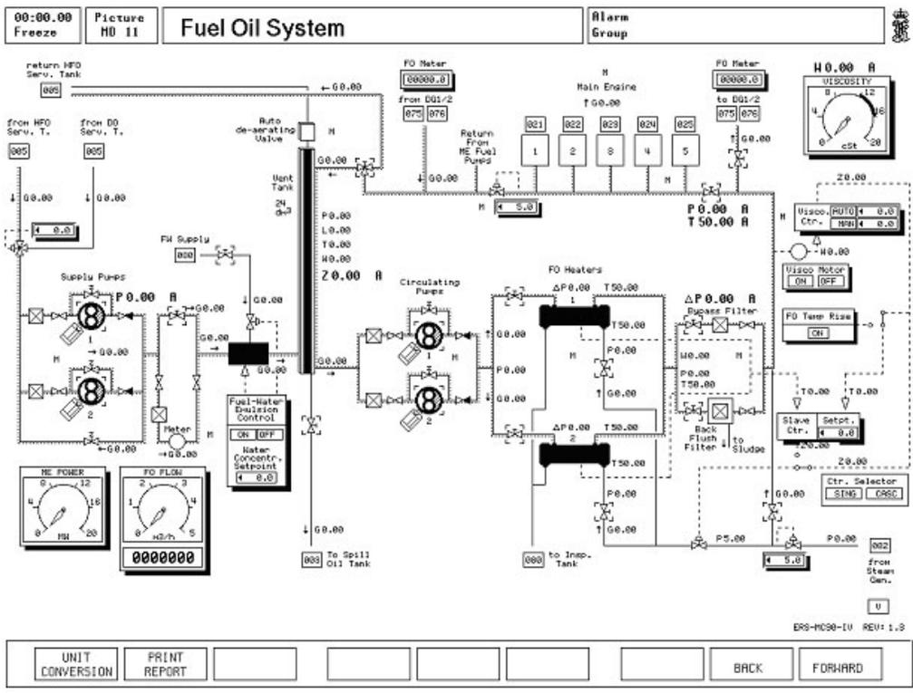
Fig. 4- Fuel Oil System with Heater and Viscosimeter (1)
