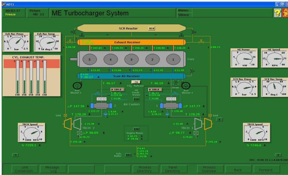
Fig. 1 – Air Cooler Heat Exchanger in Turbocharger system (1)
