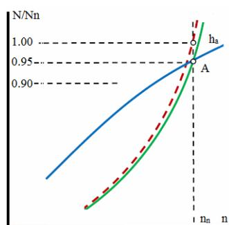
Figure 1 Combined point between Main Engine - Propeller in designing
