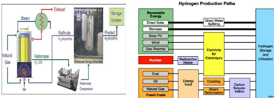
Fig. 3 left- H2 Natural Gas, steam reformer, right- H2 production path ways. Source DOE
