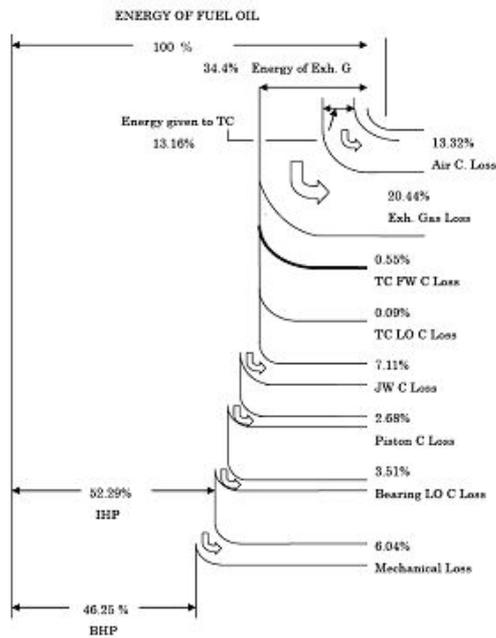
Fig. 2 Heat balance diagram II
