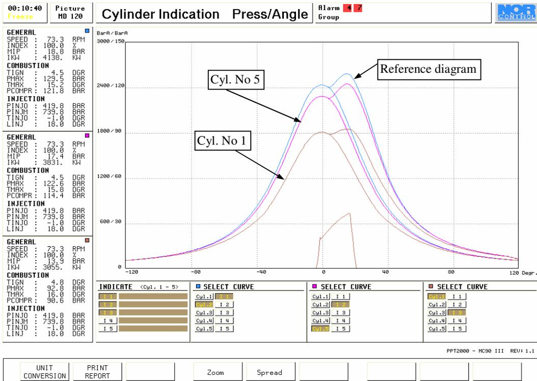
Figure 10: Cylinder Indicator Diagram
