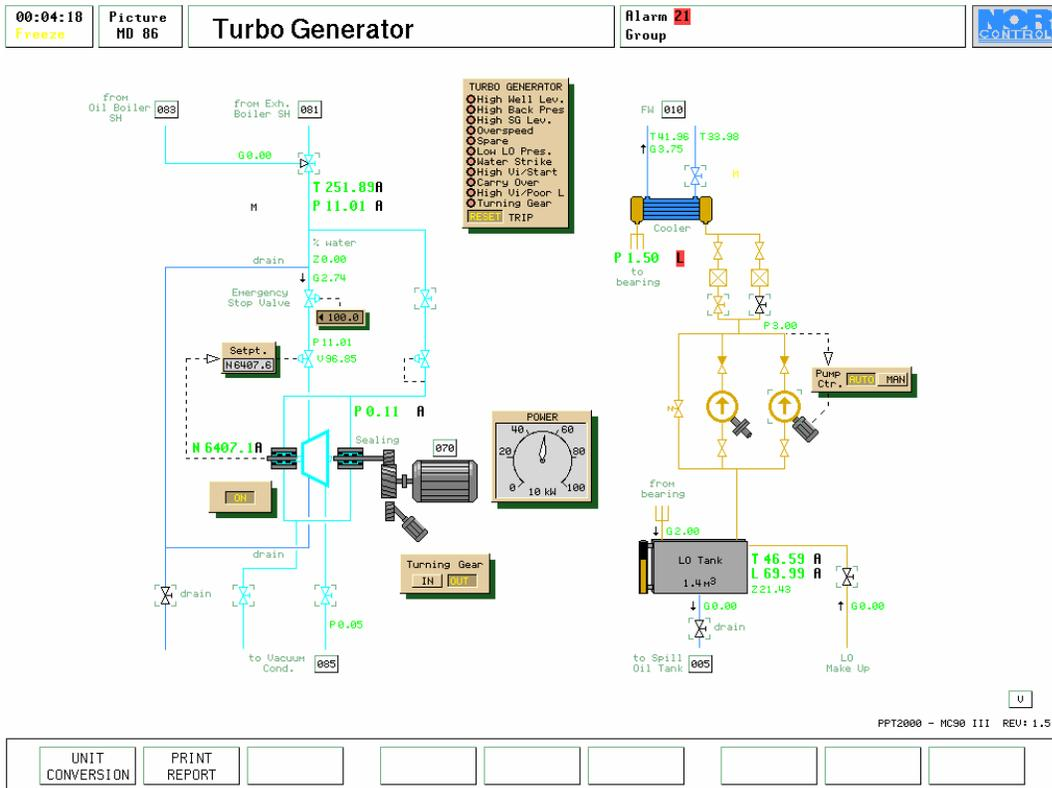
Figure 6: Turbo Generator Layout System
