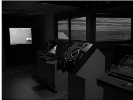
*Figure 2: 50-inch display unit of the ISSS installed in bridge mockup*
