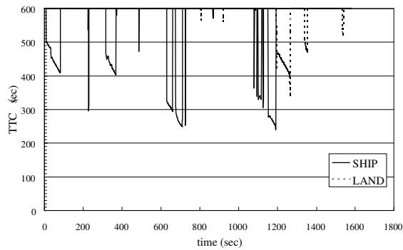
**Figure 8: An example of TTC (ship & land) result with collision avoidance maneuvers on scenario 3**
