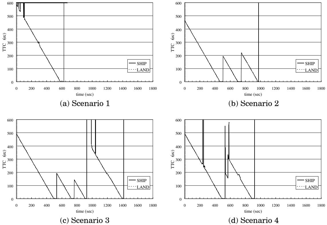
**Figure 7: TTC (ship & land) results without collision avoidance maneuvers**
