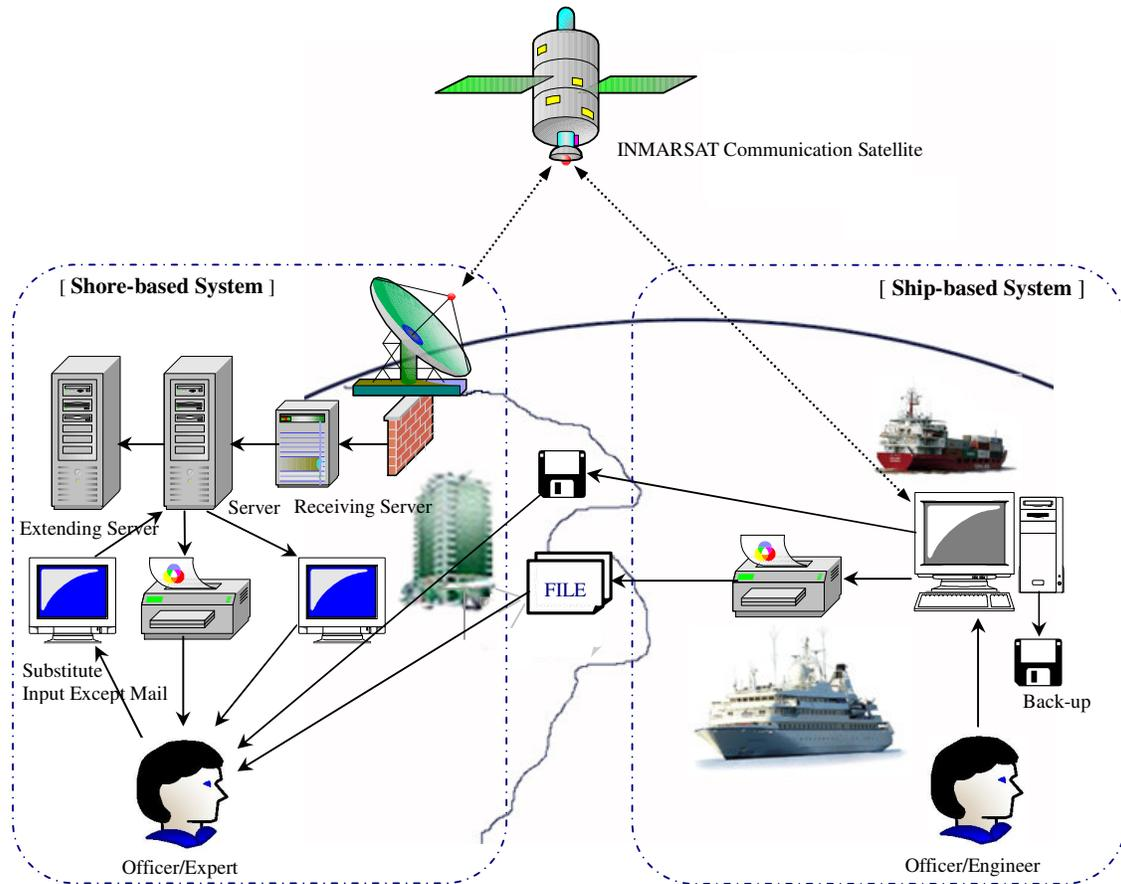
*Figure 1: System Schematic Diagram*
